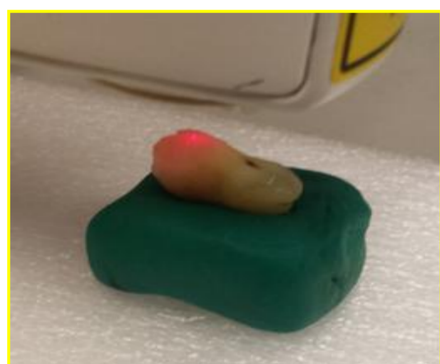
Figure 1. Tooth mounted on scanning table with centre of scanning area indicated with a fine red light
